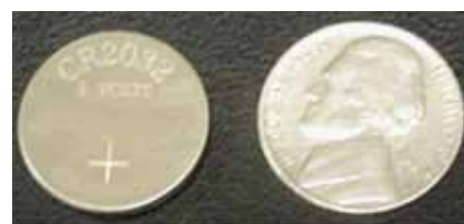
Popular sizes of 3 Volt CR or BR, 20mm Lithium cell batteries include: 2016, 2025, 2032
